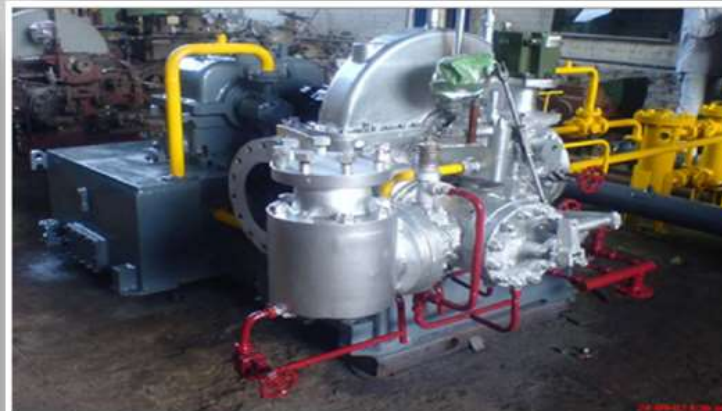
600 KW BACK PRESSURE TURBO - GENERATOR SET AT PATTOKI SUGAR MILLS, PAKISTAN (Total = 06 Installations)
