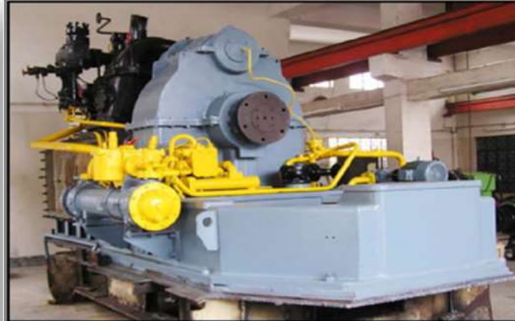
1000 KW EXTRACTION CONDENSING TURBINE - GENERATOR SET AT K. M. PAPER MILLS
