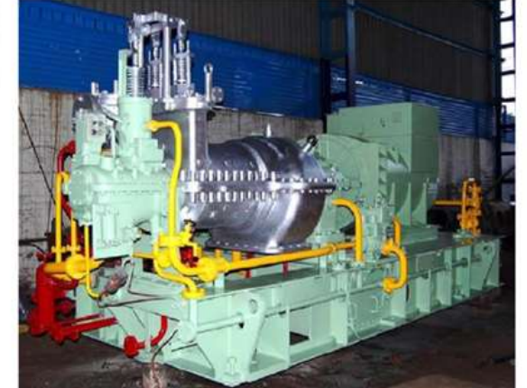
1500 KW LOW PRESSURE TURBO - GENERATOR SET AT SIDDHARTHA PAPER MILLS, (P) LTD. KASHIPUR (U. P.)
